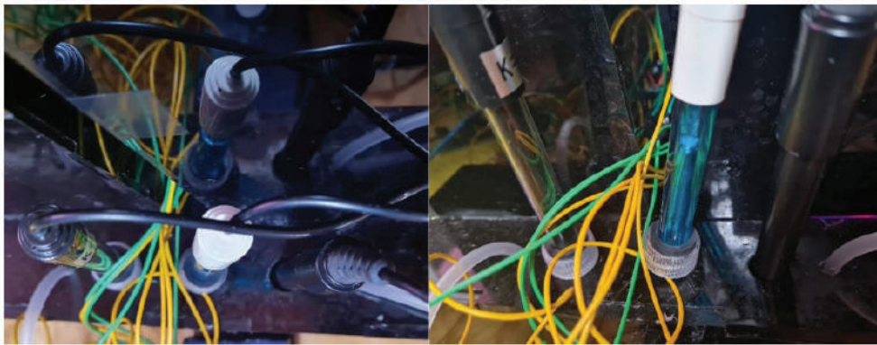
Figure 3. Mounting of pH, conductivity and oxygenation sensors in the prototype's water tank.
